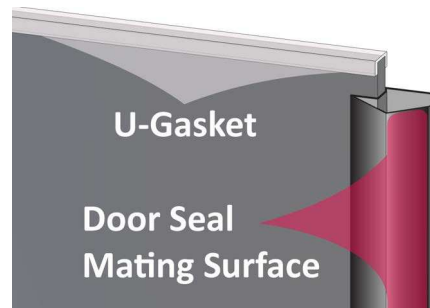
Figure 17. Single Glass Pane Orientation & U-Gasket
