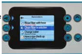
The Maintenance reminders menu allows you to verify the time left before maintenance is required, as well as to reset the time once a task is completed.
