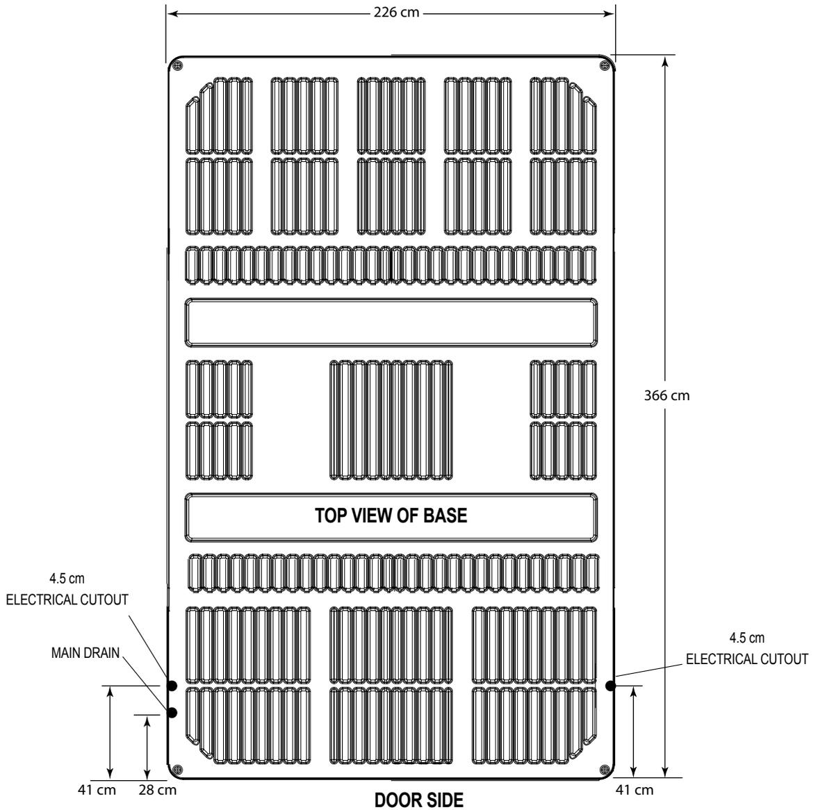
**NOTE:** ENDLESS POOLS requires that the X200 Model be installed on a minimum 15 cm thick reinforced concrete pad or structurally sound deck able to support the "dead weight" found in the specification chart on the back page.
