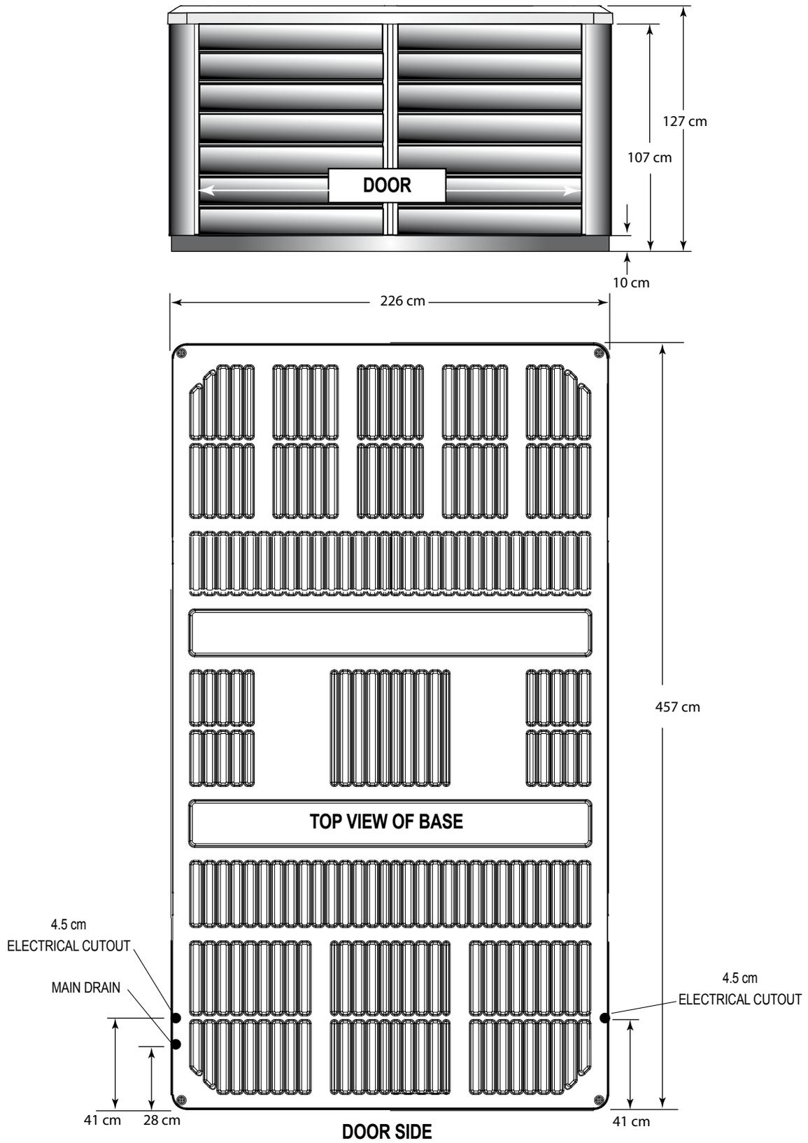
**NOTE: ENDLESS POOLS** requires that the X500 Model be installed on a minimum 15 cm thick reinforced concrete pad or structurally sound deck able to support the “dead weight” found in the specification chart on the back page.
