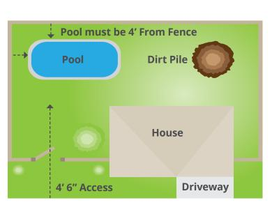
The installation crew will require the location of the plumbing equipment for the purpose of where to orient the **skimmer and return cut out.** These are pre cut in the pool walls so once the wall has been erected this location will be unable to be changed.
