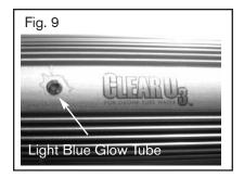
the Clear O3®. A light blue light indicates lamp is lit and the unit should be producing ozone. (Fig. 9)
