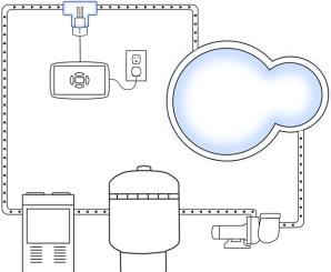
6. Replace this part of the pipe with the tee assembly and fasten with standard PVC primer and glue making sure that the direction of water flow goes between the two electrodes and the tee is always full of water.
