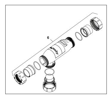
Figure 19. 3-Port Spool Exploded View
