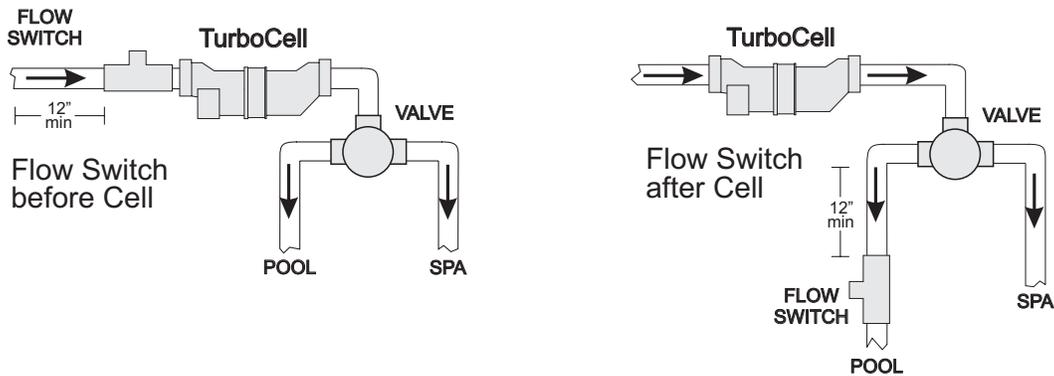
The cell may be mounted vertically or horizontally, and water can move in either direction through the cell. Install using the 2" unions provided. Tighten unions BY HAND for a watertight seal. For systems with 1½" plumbing use adapters (provided by installer).
