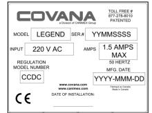
Specification label, located on the AC control box Note: This label provides the serial number (For AC operated model only, European Only)
