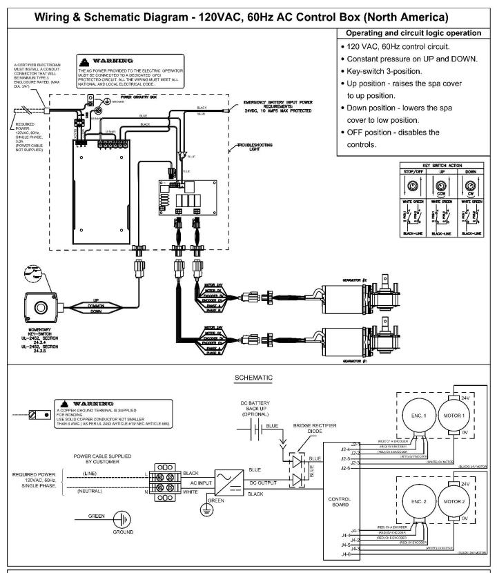
The control circuit operates at 120VAC, 60Hz. Due to the resistance in the wire used to carry the control circuit voltage, it is important to use the appropriate wire size between the AC control box and the main power supply. If wire gage is not suitable for the distance, problems in AC control box will be encountered such as motor humming, premature wear of the power supply and possible tripping of it's thermal protection.
